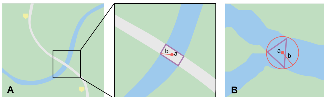
Figure 9. A: Crossing of a road and a stream with details of boundary, corrected center a (with no need for correction) and geographic radial b of the intersection. B: Boundary, corrected center a and geographic radial b of a confluence of two rivers.
